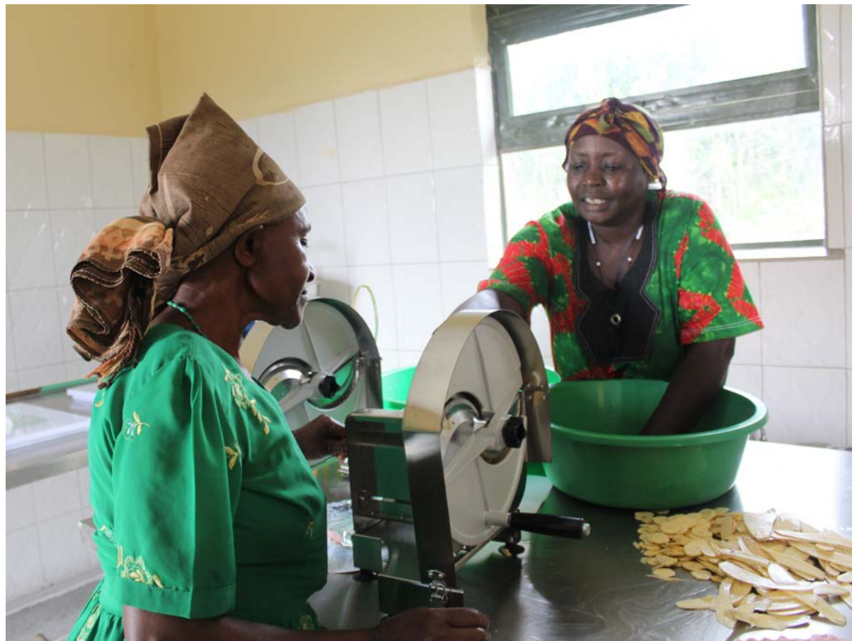
Banana processors at Rutunguru cluster farmers Association in Ntungamo district use a slicing machine donated by UNIDO to ensure high quality of banana fruits processed for the market
